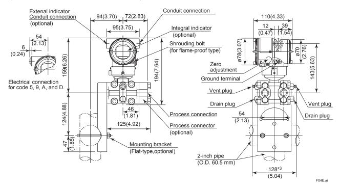
\*1: When installation code 8 is selected, high and low pressure side on above figure are reversed. (i.e. High pressure side is on the right side.)
