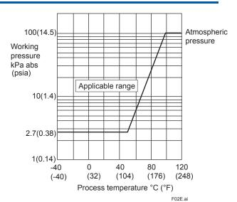
Figure 1-2. Working Pressure and Process Temperature [For EJX530A]
